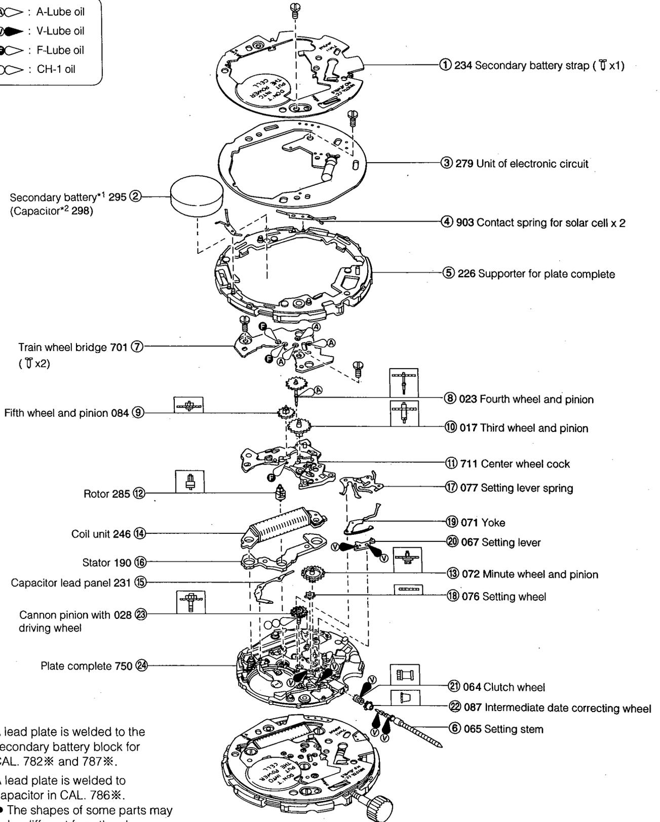
\*1: A lead plate is welded to the secondary battery block for CAL. 782\* and 787\*.
